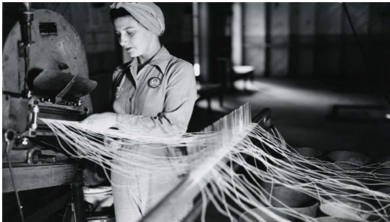
Female worker cutting powder strands at Hercules plant during World War II
